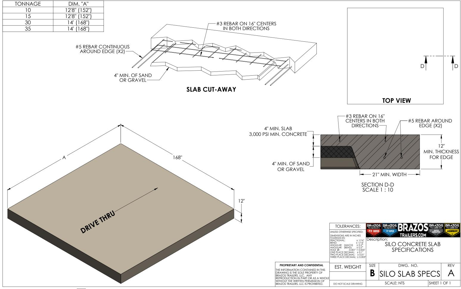
SLAB ASSEMBLY REV A
